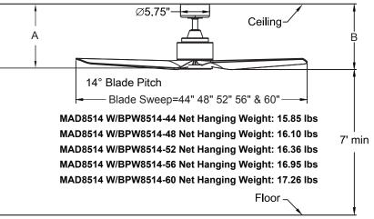
Fan must be attached to a securely anchored electrical junction box capable of withstanding a load of at least 35 lbs.
