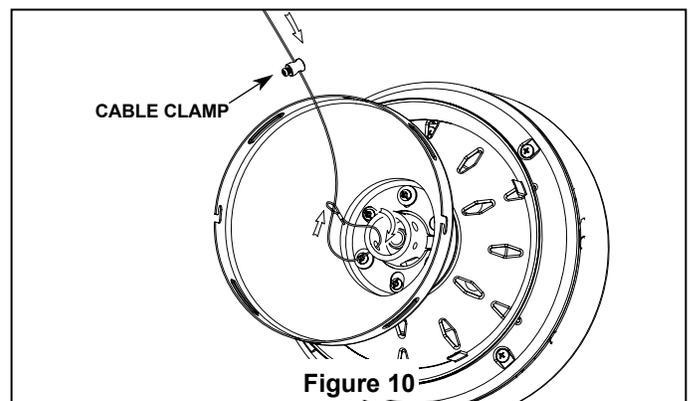
10. Loop the safety cable end through one of the holes in the hanger plate up into the outlet box, then back out the center of the plate, then connect the end with the screw down clamp. Tighten the set screw in the clamp. (Figure 11).
