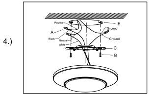
$Step \ 4. \ \ \text{Align fixture spring with cutout in mounting strap} \\ \text{and press towards mounting surface to snap into place} \ .$
