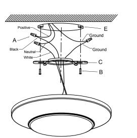
Mounting: These fixtures mount directly to most standard metallic & non-metallic electrical boxes with 2-3/4" to 3-1/2" hole spacingthat are at least 1-1/2" deep. This includes 3-1/2" & 4" octagon boxes, round mud-rings for octagon and square boxes, and 3" & 4"non-metallic round boxes. Products are suitable for mounting on ceilings or walls, and are acceptable for use within closet storage spaces when installed per NEC requirements.
